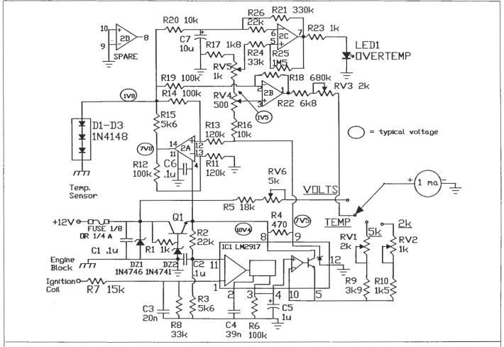
In our November issue, the schematic diagram of the Automotive Multifunction meter was less than clear because of (a) a new drafting system that deleted some of the symbols, and (b) hasty proofreading. Our apologies to the author and to readers who had difficulty with this one. The corrected schematic is shown above. Also, the various leads such as 12V, ground, sensor, etc. can be put through a multi-lead connector for convenience.
